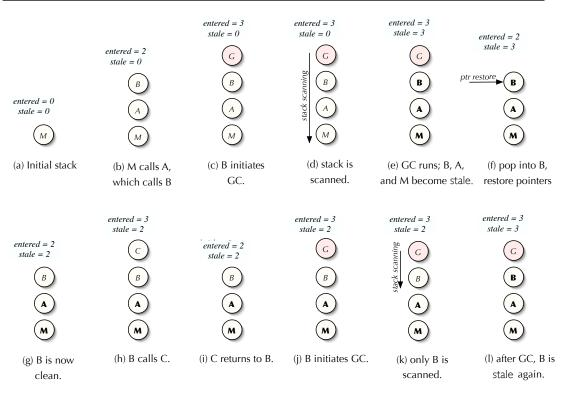
Figure 8. Example of lazy pointer stacks with pointer restoration.
